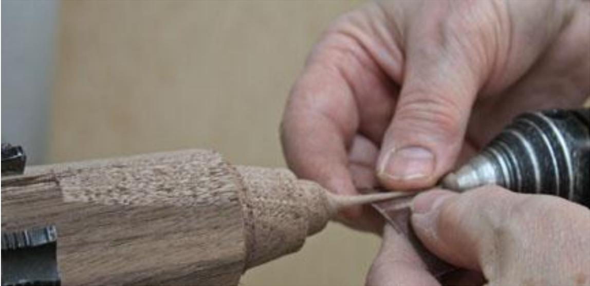
6. Sanding a completed section, supporting the stem to prevent flexing.
