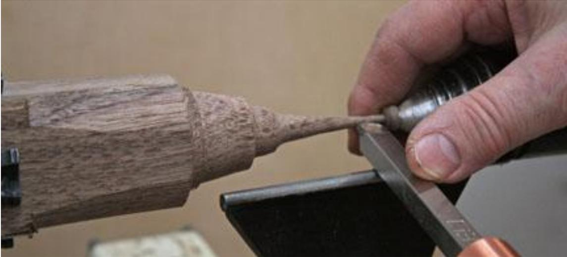
5. Working down the taper, keeping one finger behind the wood to support it.
