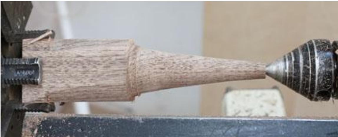
2. Blank turned with tapered cone at end.
